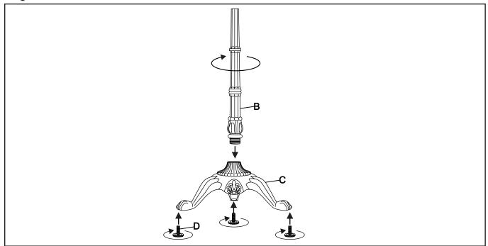
Place the base (C) on a non-marring flat surface. Align threaded end of the post (B) onto base (C) as shown above in the drawing. Rotate post (B) in clockwise direction until secured. Align and insert leveler (D) on the base. Adjust leveler (D) for balancing the base (C) as required.
