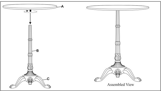
Align threaded stud of, marble top (A) onto pre-assembly (B+C). Rotate marble top (A) in clockwise direction until marble top (A) is fully secured. Assembly is complete. Product is ready to use.
